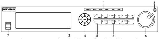
Figure 1-5 Front Panel of DS-7300HQHI-F/N and DS-7300HUHI-F/N
