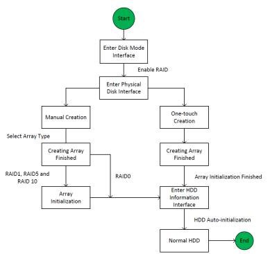
Figure 13-1 RAID Working Flow
