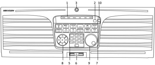
Figure 1-8 Front Panel of DS-9000HUHI-F16/N
