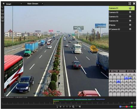
Figure 6-14 Smart Playback Interface
