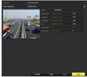
Figure 15-5 Image Settings Interface (Analog Camera)
