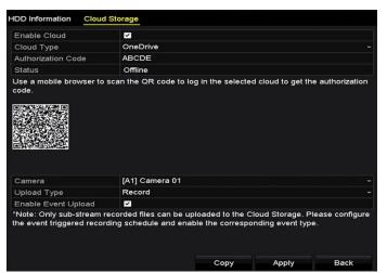
Figure 14-20 Upload to Cloud Storage Interface
