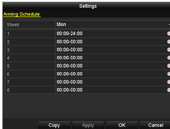
Figure 8. 24 Set Arming Schedule of Alarm Output
